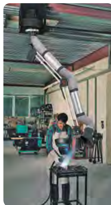
RG-200 with ball joint extraction arm
