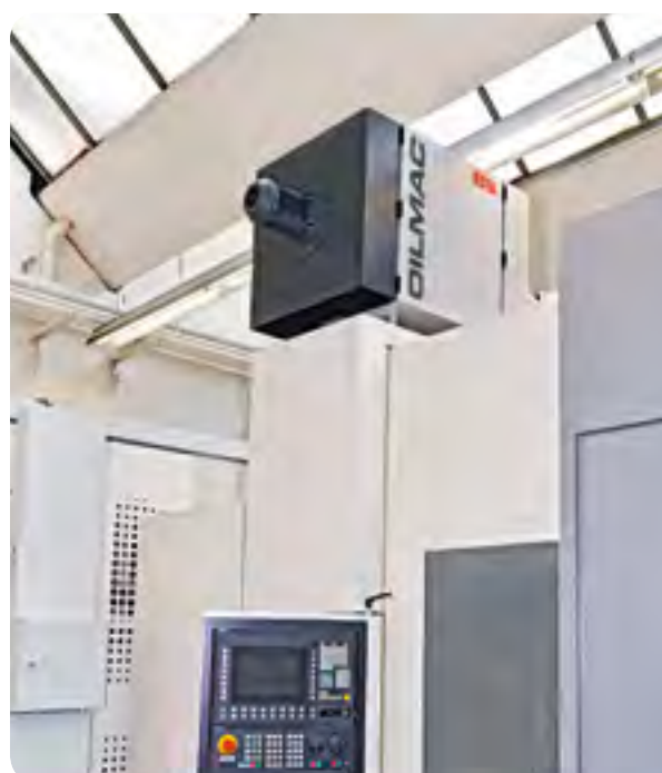
OILMAC 1600 on a processing machine
