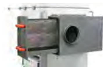
The sides of the spark pre-separator serve to dispose of residue.
