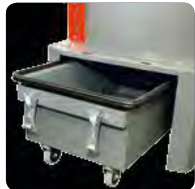
The detachable dust collection drawer makes for easy disposal of a dust
